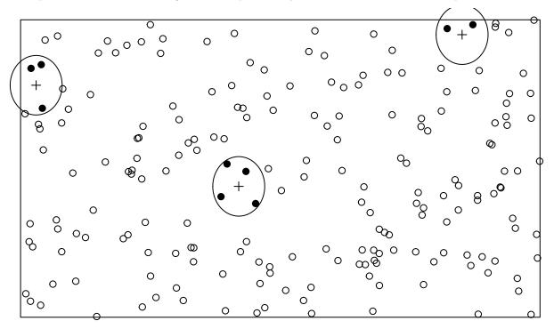
The probability that an object will be included within a plot equals the area of the plot that is also within the region when the center of the plot is centered on the object.
